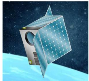
Figure 8: SEEING 10-m (or SEEING 1.8-m) implemented within a 18U Cubesat
