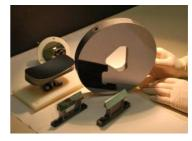
Figure 3: Safran Reosc SiC optics polished for Astroterra
