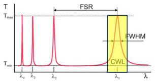
Figure 7: Limited integrated transmission of Fabry Perot filter
